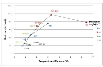
Fig. 5: Variation of heat rejected in condensing section with temperature difference
